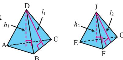
$$\frac{AB}{EF} = \frac{BC}{FG} = \frac{CA}{GE} = \frac{AD}{EJ} = \frac{BD}{FJ} = \frac{CD}{GJ} = \frac{h_1}{h_2} = \frac{l_1}{l_2} = k$$
